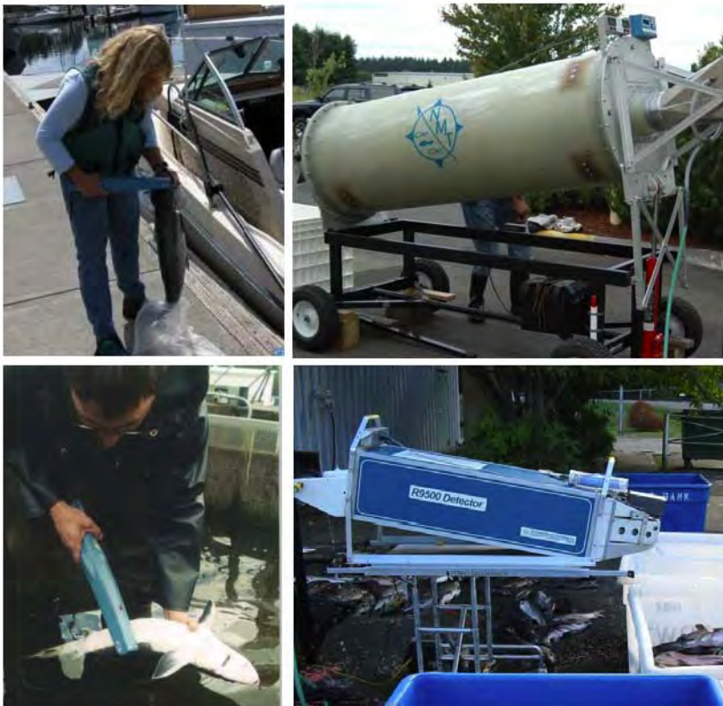
Figure 8. Electronic detection is used to sort fish with tags from those without tags in the absence of an external mark. Handheld Wand Detectors (left photos) are easily adapted to any sampling location while tunnel detectors (right photos) are more suitable for sites with large numbers of fish to be sorted.
