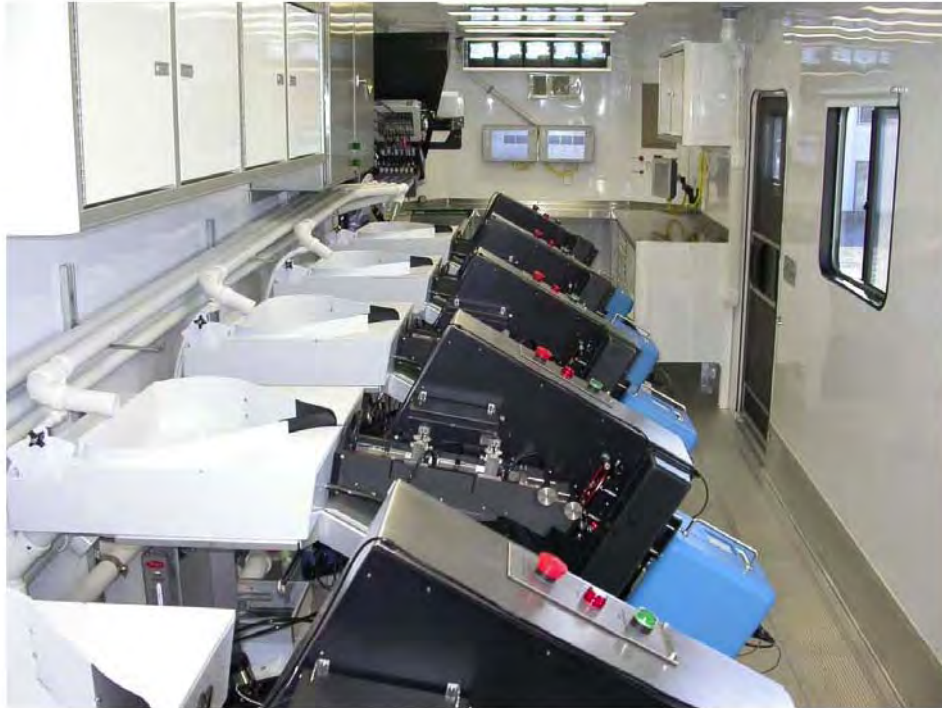
Figure 3. The main working components of AutoFish are the sorter (left, in background) and the marking and tagging lines (foreground).
