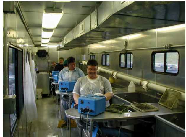
Figure 3. Interior of a manual tagging trailer using Mark IV tag injectors (photograph by George Nandor).
