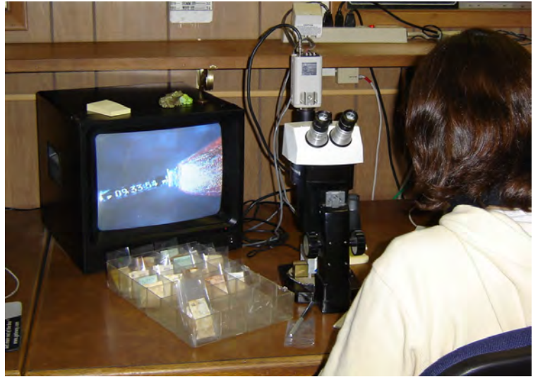
Figure 7. A recovered CWT magnified and displayed on a monitor for easy reading (photograph provided by ODFW).
