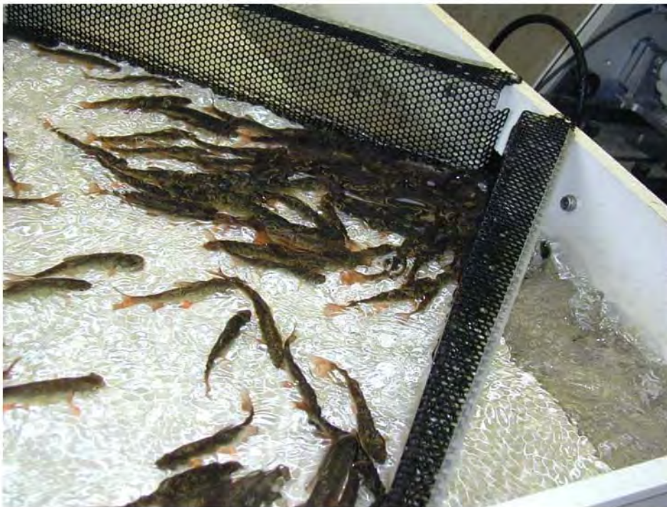
Figure 5. Fish are not anesthetized or handled by humans once they are in the trailer. AutoFish relies on Volitional Entry Devices (VE, the white trays at the top of the sorter and each marking and tagging line) to move the fish through the measuring and diverting device and the marking and tagging lines. The VE is a shallow, bright environment with upwelling water that takes advantage of the fish's natural instinct to seek a darker, more protected location, in this case, the entry to the sorter or marking and tagging line.
